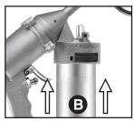
B. Push barrel into head and release
