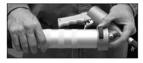
Recommended method for holding grease gun to disengage barrel.
